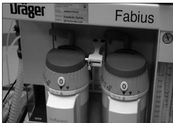
Figure 1. Note the interlocking bar between the vaporizers, that are in series
