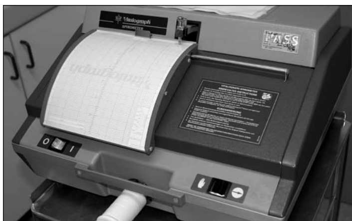
Figure 4. A vitalograph consists of a bellows attached to a pen, with a motor, which moves a sheet of paper under the pen tip, as the subject exhales and fills the bellows. A typical reading is shown in Figure 5
